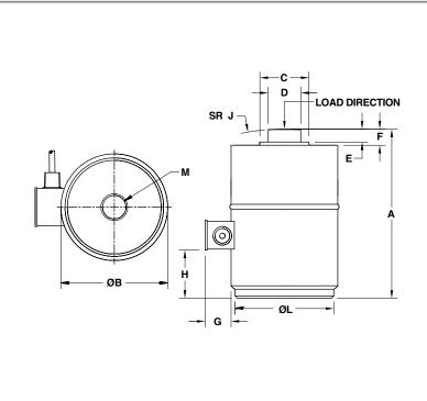
**Cable specifications** Cable length: 12.2m (40 ft) Excitation + Red Excitation -Black Output + Green Output -White Shield Transparent
