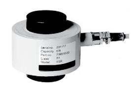
A reliable sealing and mechanical protection of the strain gage area is ensured by the use of stainless steel diaphragms and a housing which are cemented to the measuring element.
